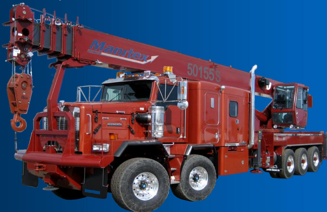
MANITEX 50155 50-TON CRANE 9,000 LB CAPACITY AT MAX TIP HEIGHT OF 165'
