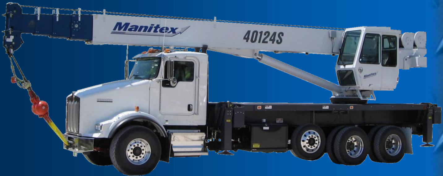
MANITEX 40124 40-TON CRANE 8,450 LB CAPACITY AT MAX TIP HEIGHT OF 132'4"
