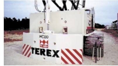
Hydraulic removable counterweight system
