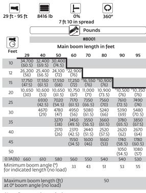
Note: Boom angles are in degrees. #LMI operating code. Refer to LMI manual for operating instructions \*This capacity is based on maximum boom angle
