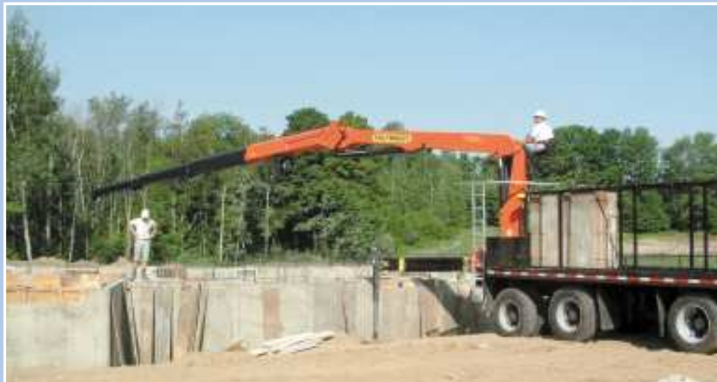
PowerLink™ linkage system gives the outer boom added strength in flat-out position and a constant folding speed.
